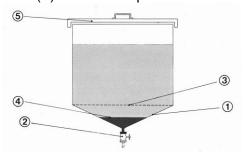
It is advisable to place the pieces to be treated inside a metal basket, which must remain above the water level (to avoid contact of the pieces with the water itself).
